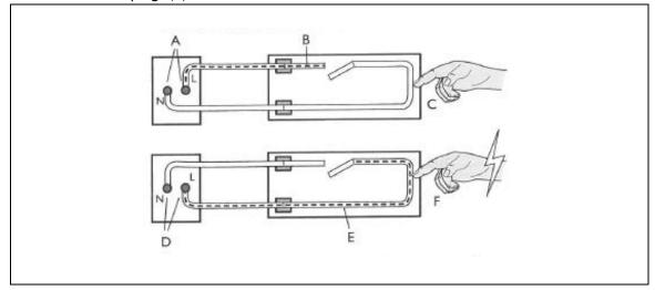
8. Fuses are connected in the live part of the circuit. If too great a current passes through them, they "blow". Label the diagram below to show how they work. (2)
