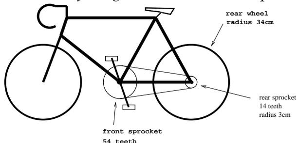
A fixed gear means that there is no freewheel: the rear sprocket is attached directly to the rear wheel, so that if the wheel turns, the rear sprocket (and hence the front sprocket and pedals) turns. You can't "coast" on such a bike. These kinds of bikes are standard in track racing. They also have no brakes, to make it difficult to make sudden speed changes. This *improves* safety in the close quarters of track racing.
