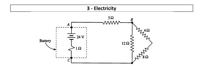
A battery with an *emf* of 24 volts and an internal resistance of 1  $\Omega$  is connected to an external circuit as shown above. Determine each of the following:
