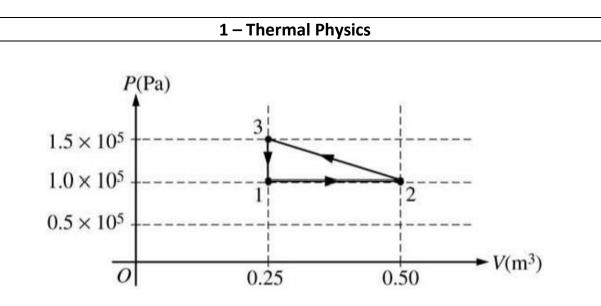
A cylinder with a movable frictionless piston contains an ideal gas that is initially in state 1 at  $1 \times 10^5$  Pa, 373 K, and 0.25 m<sup>3</sup>. The gas is taken through a reversible thermodynamic cycle as shown in the *PV* diagram above.
