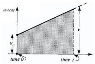
The diagram above shows a body in motion with constant acceleration. Its velocity changes in a regular way from  $v_0$  to  $v_1$  in a time t – it is a straight-line (linear) graph.
