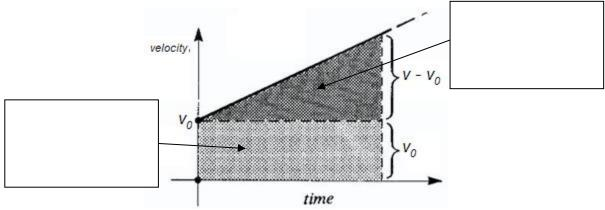
The total displacement of a body moving in a straight line with constant acceleration can be found from the area under the graph.
