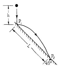
A ball of mass m is released from rest at a distance h above a frictionless plane inclined at an angle of 45° to the horizontal as shown above. The ball bounces horizontally off the plane at point  $P_1$  with the same speed with which it struck the plane and strikes the plane again at point  $P_2$ . In terms of g and h determine each of the following quantities:
